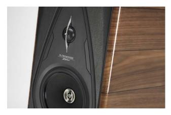
Sonus faber refers to its tweeter as an Arrow Point Damped Apex Dome, which is 28mm (1.1 inches) in diameter and handles the audio spectrum of 2,500 Hz and above. Designed by Sonus faber, the driver has a neodymium motor, which creates linearity. A mechanical interface helps decouple the tweeter from the cabinet; it sits in its own complicated maze-like wood enclosure, furtherenhancing its flat frequency response.
