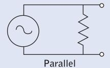
This diagram shows how the RPGC Parallel devices are wired. There is no added resistance or impedance, so the dynamics of your system are fully revealed.
