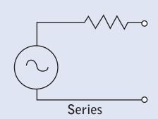
The above diagram shows how a series device is wired. This method increases impedance and limits current since electricity has to pass through thousands of feet of wire along with other components that add resistance.
